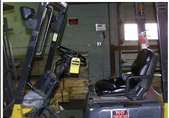
Yellow Tag without a Lock non-energized equipment out of service
